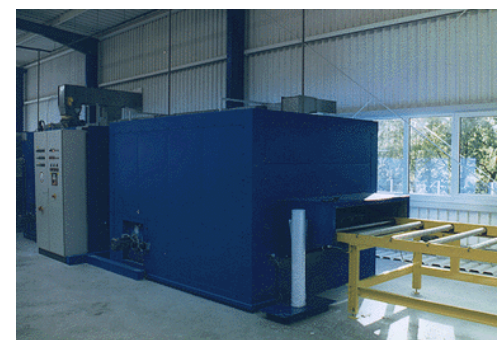
Drying oven for coated corrugated sheet metal
